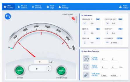
Control System HMI
